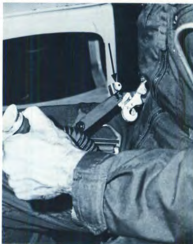
One tug on the hose and the right leg fastener releases the leg strap.
