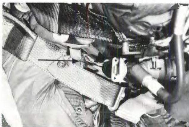
The oxygen hose restraining strap became entangled in the release mechanism of the right leg fastener of the parachute.
