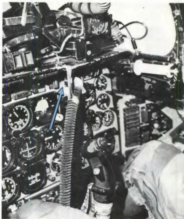
After flight, oxygen hose is stowed here by clipping the restraining strap on the instrument shroud.
