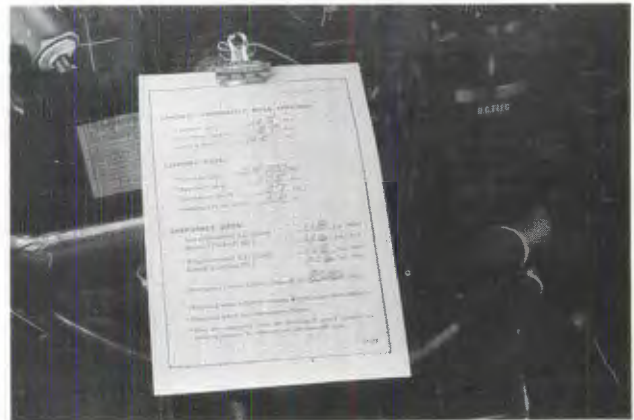
The TOLD card was blocking the pilot's view.
